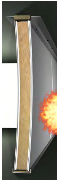
Figure 15. The behaviour of PAROC panels in fire.
